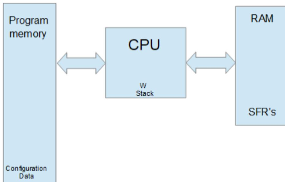
Note that the buses on each side of the above diagram are different data width sizes. On the left, is 12,14,16 or 24 bits depending on the PIC® MCU. On the right it is 8 or 16 bit. One advantage to this architecture is both memory spaces can be accessed at the same time.
